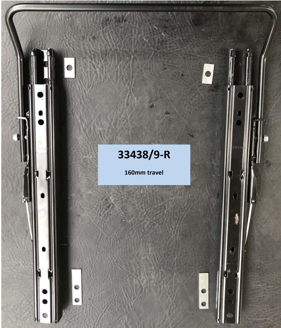
These sliders can be fitted to one of two Chapman fixed plinths designed specifically for the R14 type seat-belted seat. If these are fitted to Optare vehicles, we have supplied the seats to them without plinths and you will need to use the bus builder's own fixing points for these sliders.
