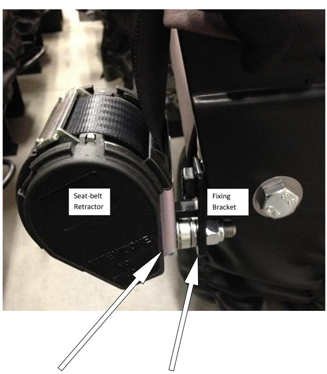
Retractor bracket should be parallel with the fixing bracket to ensure that the belt releases vertically. If the retractor is knocked or fouls on the vehicle bulkhead, this can cause the belt to "stick" and not operate smoothly. If the bracket is not feeding the belt at 90 degrees to the floor, this can usually be rectified by bending the retractor back into position.
